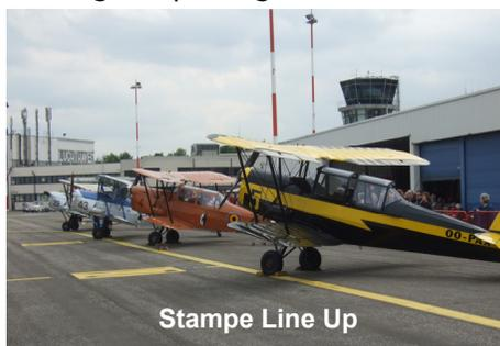
In total 940 of the Stampe or SV.4 were built; it was designed by George Ivanov and built by Stampe et Vertongen near to Antwerp. At a quick glance it looks like a Tiger Moth but I am told it is a superior aircraft with better handling.
